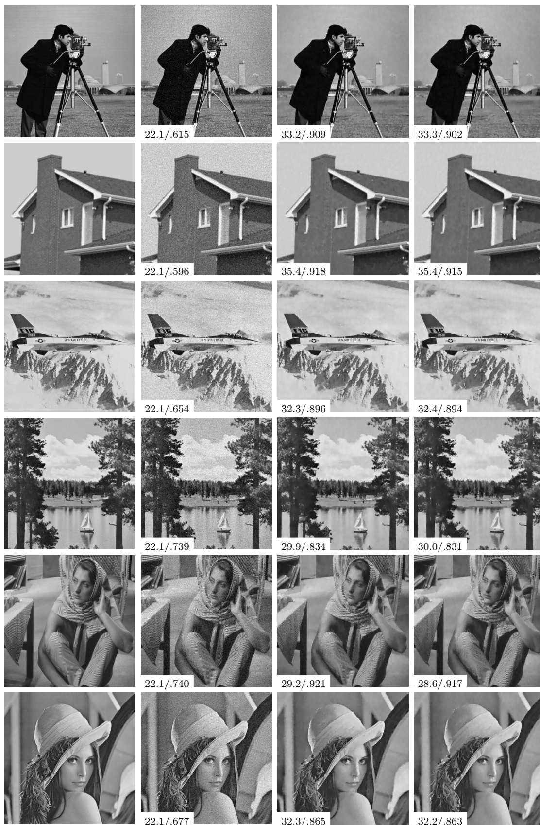
Figure 4. From left to right: Original images, noisy images with noise \sigma^2 = 20 , results with EM model, results with LR-COMP model. The denoising results are evaluated with PSNR/SSIM. Similar denoising performances are obtained with LR-COMP with a 1000 times smaller compressed database. To estimate the prior model, our method is 2 times faster than the EM algorithm.
