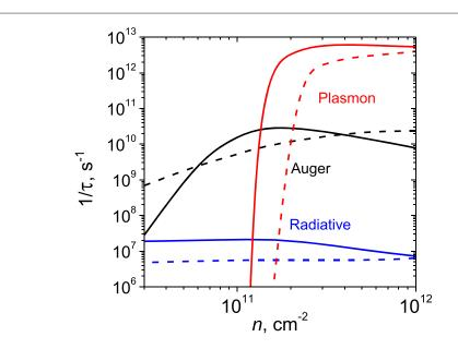
**Figure 6.** Dependences of the recombination frequency (inverse lifetime) on the concentration of nonequilibrium carriers for three recombination mechanisms in 5-nm-wide HgTe QW. Solid lines correspond to the effective carrier temperature 4.2 K, dashed ones—to that of 77 K. Lattice temperature is 4.2 K.
