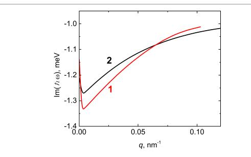
**Figure 4.** Calculated dependences of the imaginary part of the plasmon energy on the wave vector for  $\hbar\nu_e = 1 \text{ meV}$ ,  $\hbar\nu_h = 2 \text{ meV}$ .  $T = T^* = 4.2 \text{ K}$ , n = p,  $\text{cm}^{-2}$ :  $10^{11}$  (1),  $2^*$  10<sup>11</sup> (2).
