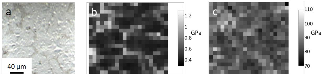
**Figure 6.** (a) Optical microscopy image, corresponding (b) hardness and (c) elastic modulus of a 0.8%  $\text{HfB}_2$ -Al nanocomposite measured with nanoindentation,  $1\ \mu\text{m}$  indents. Black pixels at 0 GPa in (b) and (c) correspond to micropores ascribed to the removal of nanoparticles during polishing.
