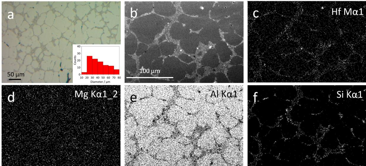
**Figure 5.** Microscopy study of a 0.8 vol%  $\text{HfB}_2$ - $\text{AlSi}_7\text{Mg}_{0.3}\text{Cu}_{0.5}$  nanocomposite prepared by ultrasound treatment with a Nb tip for 5 minutes and cooled down in liquid nitrogen. (a) Optical microscopy image and corresponding size distribution of Al grains, (b) SEM micrograph and (c-f) corresponding SEM-EDS maps. The scales are identical from (b) to (f).
