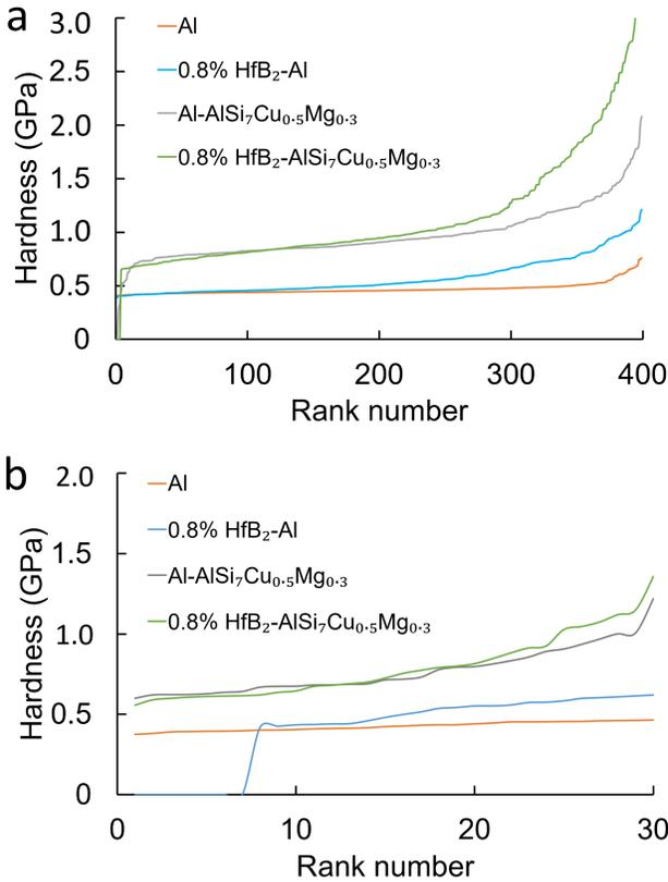
**Figure 7.** Statistic evaluation of hardness measured at 1  $\mu\text{m}$  (a) and 3  $\mu\text{m}$  (b) for reference Al and Al-AlSi<sub>7</sub>Mg<sub>0.3</sub>Cu<sub>0.5</sub> samples, for the 0.8 vol.% HfB<sub>2</sub>-Al and HfB<sub>2</sub>-Al-AlSi<sub>7</sub>Mg<sub>0.3</sub>Cu<sub>0.5</sub> nanocomposites.
