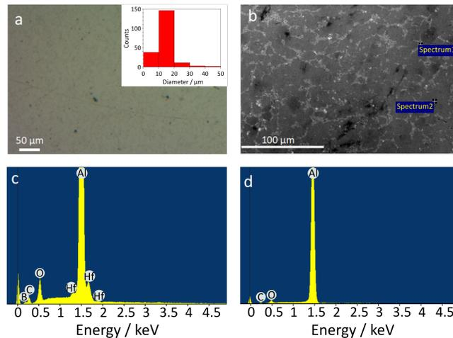
**Figure 3.** Characterization of a 0.8 vol%  $\text{HfB}_2$ -Al nanocomposite prepared with ultrasound treatment with a Nb tip for 5 min. and cooled down in liquid nitrogen. (a) Optical image and size distribution of Al grains. (b) backscattered SEM image and corresponding EDS analyses of (c) a
