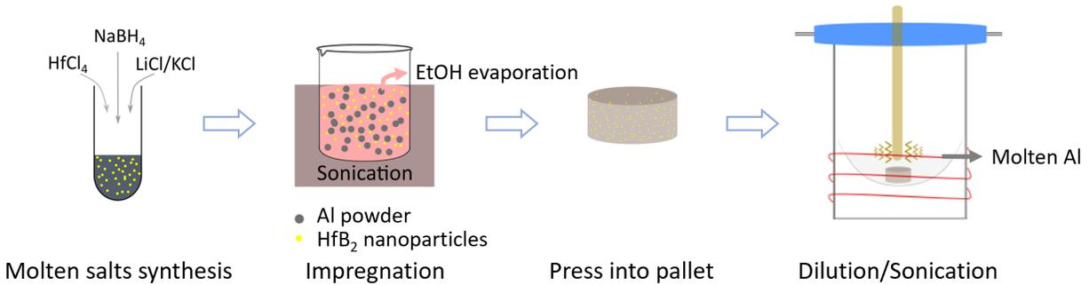
**Figure 1.** Scheme of the synthesis procedures of HfB<sub>2</sub>-Al nanocomposite
