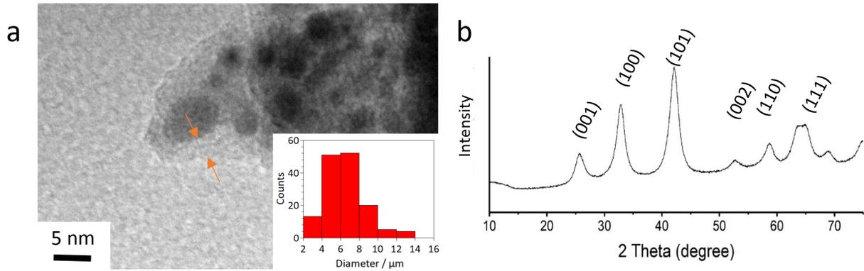
**Figure 2.** (a) TEM image and (b) powder XRD pattern (indexed along the HfB<sub>2</sub> structure) of HfB<sub>2</sub> nanoparticles coated with an amorphous boron-rich layer, as shown between two arrows.
