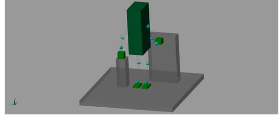
Fig. 2. Starting posture of the robot, making 4 contacts with the environment.
