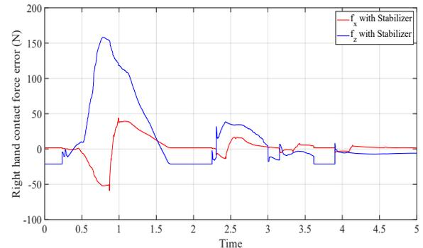
Fig. 6. The x and z components of the contact force error at the right hand when using the Stabilizer, in the case of multiple perturbations
