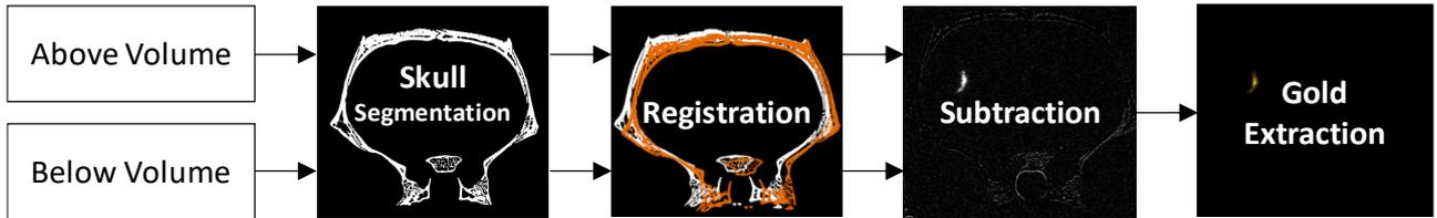
Figure 2. The 4 steps of the cells tracking pipeline resulting in a map of gold concentrations obtained from the two volumes acquired above and below the gold K-edge.
