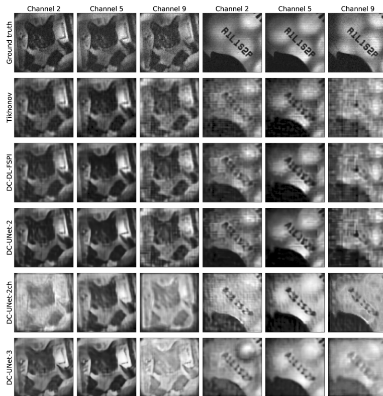
Fig. 3. Reconstruction of the experimental acquisition of two objects: STL-10 cat (columns 1–3) and off-centered Siemens star (columns 4–6). The top row displays the ground truth images for the 2nd, 5th and 9th channels. We compare the reconstruction results using five methods: Tikhonov, DC-DL-FSPI, DC-UNet-2, DC-UNet-2ch, DC-UNet-3.
