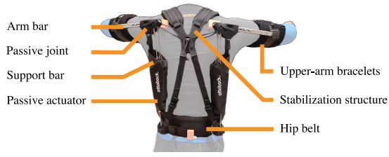
Fig. 2: Ottobock PAEXO assistive passive exoskeleton.
