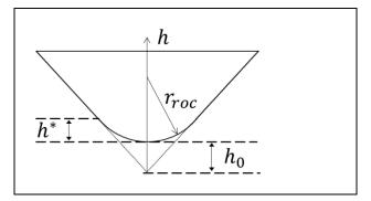
Figure 3: Schematic description of tip defect.
