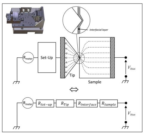
Figure 5: Schematic of the individual contributions to the measured resistance and the corresponding electrical cicruit. Dotted lines represent the current lines.
