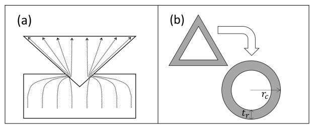
Figure 6: Schematic of current line distributions. (a) Vertical cross-section of current constriction at contact periphery. (b) Horizontal cross-section: conversion of the actual triangular cross-section into a circular ring-shaped cross-section (suitable for axisymmetric numerical modeling).
