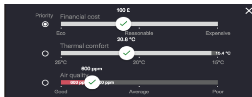
Fig. 18. The TOP-Sliders allow users to find the best tradeoff between conflicting criteria, financial cost, thermal comfort, and air quality.
