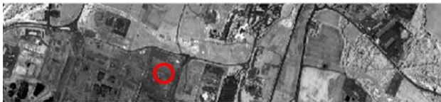
Figure 3. Hyperspectral radiance image acquired with HySpex-NEO camera and plotted at 967 nm. The circle represents the emission point.
