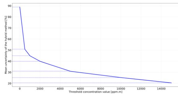
**Figure 14.** Uncertainty of the hybrid method for the real data as a function of the threshold concentration value use to calculate the mean uncertainty, in percentage.
