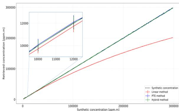
**Figure 5.** Retrieved concentrations for the three methods according to the synthetic plume concentration in brick full-synthetic case. A zoom between 9500 and 12500 ppm.m is overplotted in the insert of this figure.
