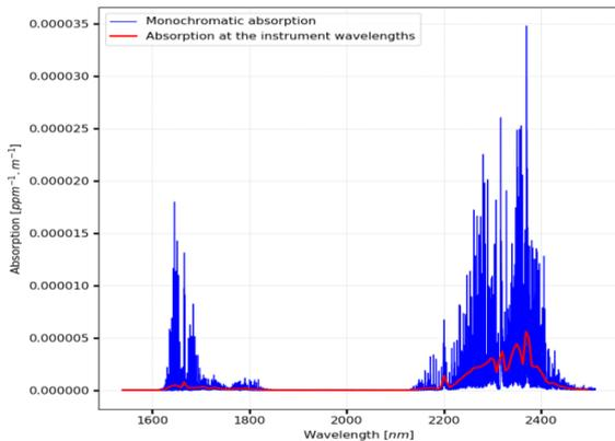
**Figure 1.** Methane monochromatic absorption in  $ppm^{-1}.m^{-1}$  of the database (Sharpe, 2004) in blue line and the methane absorption in  $ppm^{-1}.m^{-1}$  convolved by the spectral sensitivity of the hyperspectral instrument in red line.
