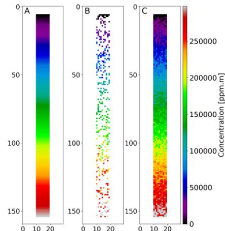
**Figure 6.** Map concentration of plume in ppm.m. Panel A: synthetic concentration. Panel B: PTE concentration. Panel C: hybrid concentration.
