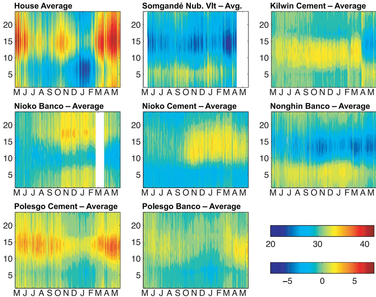
335 **Figure 4** Daily vs. hourly indoor temperature diagrams for the recording period between 25 April 2017 and 22 May 2018. Upper left-hand diagram: average of hourly indoor temperatures (°C, upper colour legend). All other diagrams: indoor temperature differences between each house and the average (°C, lower colour legend).
