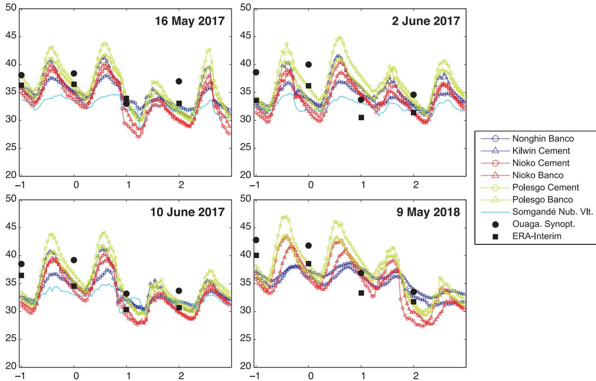
**Figure 9** Illustration of four (out of 12) selected abrupt decreases in Tx. Black dots: day-to-day changes in Tx according to the Ouagadougou synoptic station (used to detect largest Tx changes). Abrupt changes occur between  $d_0$  and  $d_1$ . Black squares: the same for ERA-Interim. Colour curves: hourly indoor temperature records in the seven houses.
