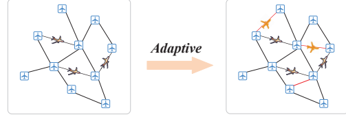
Fig. 3. Illustration of the evolution of the graph convolution operator. Blue point: civil airport. Black line: the scheduled air routes. Red line: the unknown temporary air routes.
