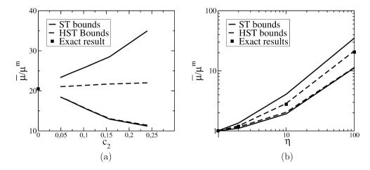
Fig. 2. (a) Overall modulus of the unit cell as a function of the volume fraction of interphase elements (contrast  $\eta = 100$ ): new bounds (HST) are compared to Hill's (ST) ones. The exact result is also reported (the filled square at  $c_2 = 0$ ); (b) Overall modulus of the unit cell (crude free mesh) as a function of the contrast (logarithmic scales): new bounds (HST) are compared to Hill's ones (ST) and to exact results (the filled squares).
