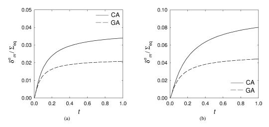
Fig. 5. Normalised stress fluctuation within the matrix estimated by the classical and generalised affine procedures for (a) aligned-fiber and (b) spherical inclusions. Same material and loading condition as Fig. 3.
