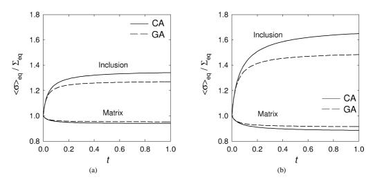
Fig. 4. Normalised equivalent average stresses per phase estimated by the classical and generalised affine procedures for (a) aligned-fiber and (b) spherical inclusions. Same material and loading condition as Fig. 3.
