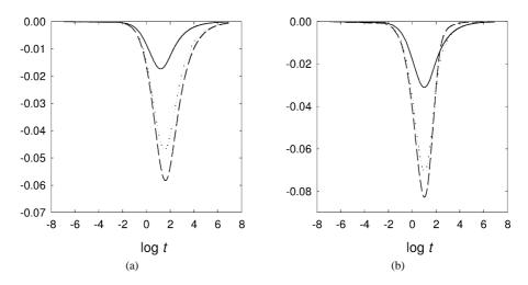
Fig. 2. Relative error between analytic and "direct" inverse transforms of (a) the average stress field and (b) the second moment of the equivalent stress in the matrix as a function of log t (continuous:  $\tau_1/\tau_2 = 2$ , dotted:  $\tau_1/\tau_2 = 10$ , dashed:  $\tau_1/\tau_2 = 100$ ).
