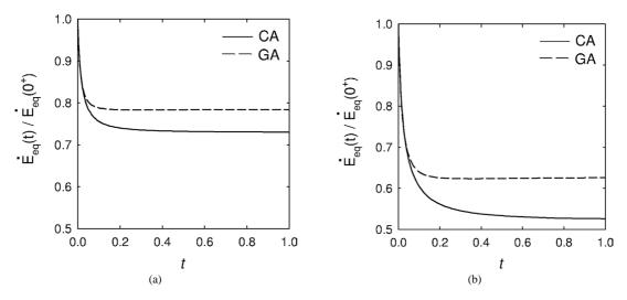
Fig. 3. Normalised overall equivalent strain rate estimated by the classical and generalised affine procedures for (a) aligned-fiber and (b) spherical inclusions. The dotted line corresponds to a decoupled Maxwell-type approach using the generalised affine procedure. The volumic fraction of inclusions is  $c_i = 0.15$  and the stress sensitivity exponent of the matrix is n = 5. Case of a longitudinal simple shear with  $\Sigma_{13}/\sigma_0^{(2)} = 1$ .
