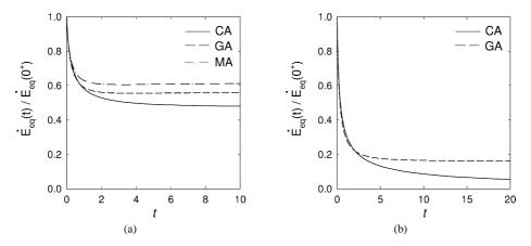
Fig. 7. Normalised overall equivalent strain rate estimated by the classical and generalised affine procedures for (a) spherical and (b) oblate ellipsoidal inclusions. The volumic fraction of inclusions is  $c_i = 0.15$  and the stress sensitivity exponent of the matrix is n = 5. Case of uniaxial tension with  $\Sigma_{33}/\sigma_0^{(2)} = 1$ .
