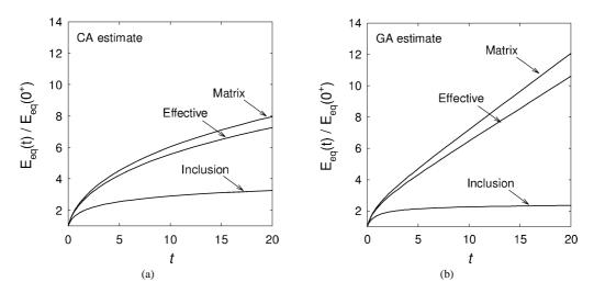
Fig. 9. Normalised equivalent average strain per phase estimated by the (a) classical and (b) generalised affine procedures for oblate ellipsoidal inclusions. Same material and loading condition as Fig. 7.
