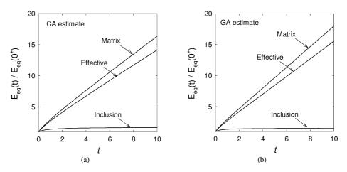
Fig. 8. Normalised equivalent average strain per phase estimated by the (a) classical and (b) generalised affine procedures for spherical inclusions. Same material and loading condition as Fig. 7.
