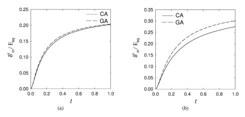
Fig. 6. Normalised strain fluctuation within the matrix estimated by the classical and generalised affine procedures for (a) aligned-fiber and (b) spherical inclusions. Same material and loading condition as Fig. 3.
