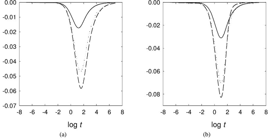
Fig. 2. Relative error between analytic and “direct” inverse transforms of (a) the average stress field and (b) the second moment of the equivalent stress in the matrix as a function of  $\log t$  (continuous:  $\tau_1/\tau_2 = 2$ , dotted:  $\tau_1/\tau_2 = 10$ , dashed:  $\tau_1/\tau_2 = 100$ ).
