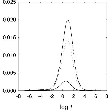
Fig. 1. Relative error between analytic and “direct” inverse transforms of the overall creep function as a function of  $\log t$  (continuous:  $\tau_1/\tau_2 = 2$ , dotted:  $\tau_1/\tau_2 = 10$ , dashed:  $\tau_1/\tau_2 = 100$ ).
