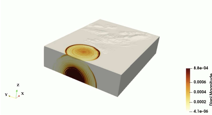
Fig. 9: Snapshot of seismic source modelled by a point-wise double-couple of a magnitude M_w 4.6 located at 14 km depth.
