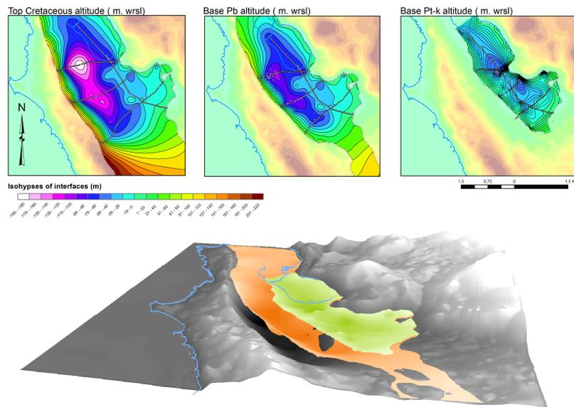
Fig. 15: Studied area. 3D refined geological model of Argostoli region is proposed by [Cushing et al. \(2019\)](#). The three top figures describe the identified three geological layers and their altitude. The bottom figure shows a 3D view of these three geological layers.
