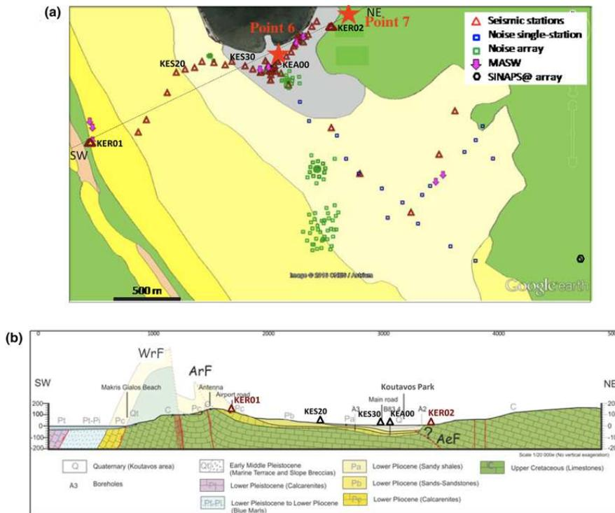
Fig. 3: (a) Plan view of the Argostoli basin together with the seismic array configuration. Contour lines of the geological map correspond to Quaternary (grey), Calcarenites (yellow), Sands-Sandstones (light yellow), Limestones (green), Miocene formation (pink) and they have been constrained using field data (NERA Deliverable D11.3). (b) geological cross-section across the basin (Hollender et al., 2015).
