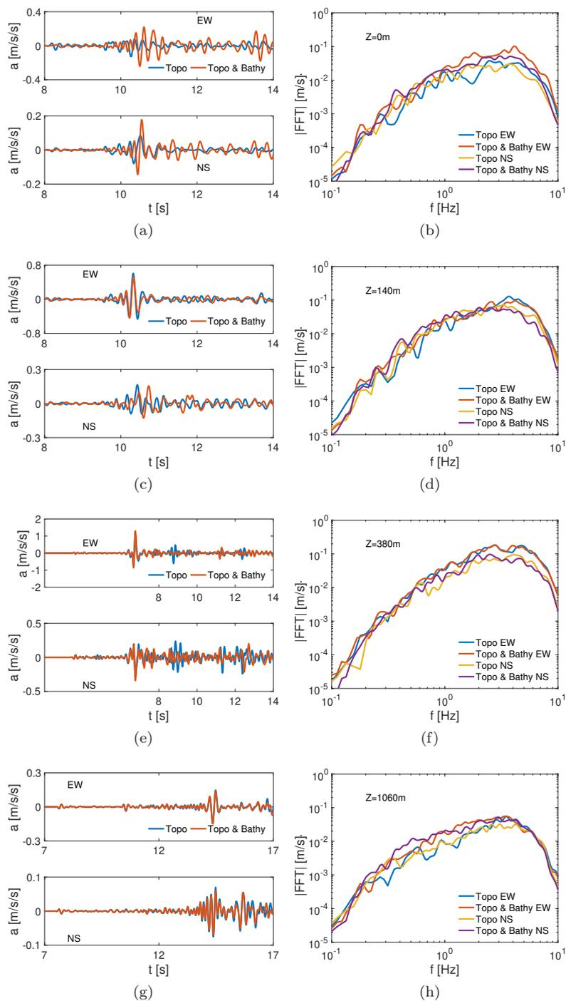
Fig. 17: Comparison of time history acceleration (a,c,e and g) and Fourier spectra (b,d,f and h) of the layered model, model including topography and the model including topography and bathymetry at the stations described in Figure 12.
