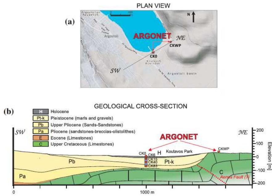
Fig. 20: Basin plan view. Line SW-NE on (a) marks the surface projection of the (d) geological cross section. Location of the registration stations of the Argostoli site are shown on the figure. The four stations are at the same point but at different depths (0, 15, 40 and 83 meters). From [Theodoulidis et al. \(2018\)](#)
