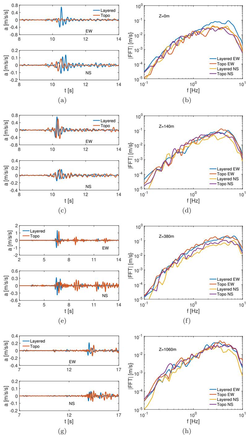
Fig. 16: Comparison of time history acceleration (a,c,e and g) and Fourier spectra (b,d,f and h) of the layered model and model including topography at the stations described in Figure 12.
