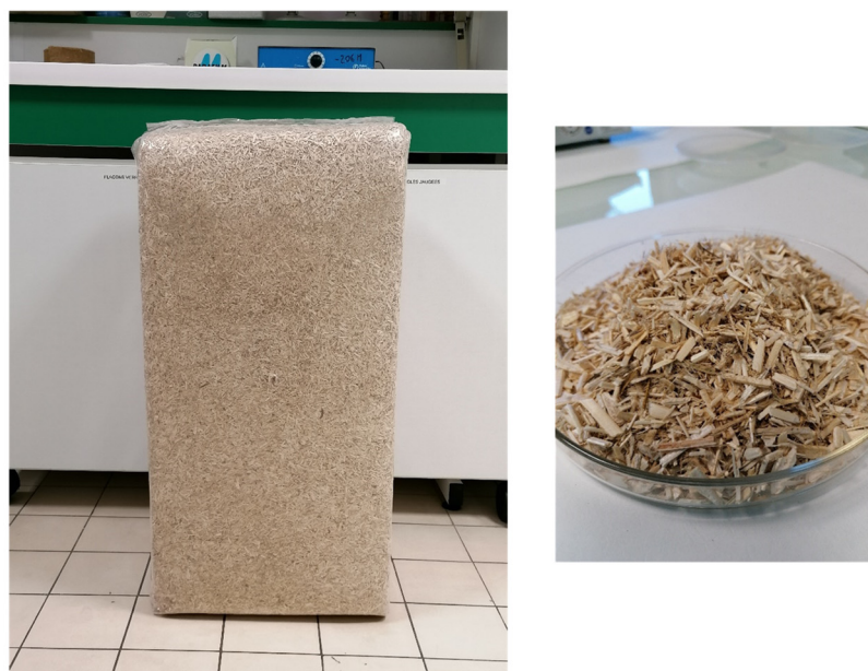
Figure 1. Chènevotte or hemp shives from a French agricultural cooperative (Eurochanvre, Arc-les-Gray, France).
