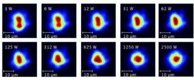
Fig. 4. Near field intensity patterns at the GRIN-MMF output recorded for increasing inputpeak powers, for appropriate settings of the input coupling, to get the self-selection of a LP01 mode.
