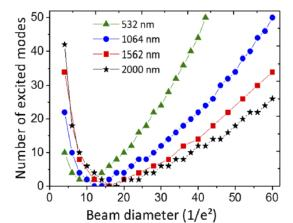
Fig. 3. Number of excited radial scalar modes (with more than 99% of input beam energy) vs. input beam diameter for four different input wavelengths.
