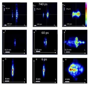
**Fig. 1.** Spectrograms (intensity vs. transverse coordinate x and wavelength \_) in the near field at the GRIN-MMF output, as a function of the output power (from left to right, 10 W, 1 kW, and 45 kW, respectively) and input pulse width (from top to bottom), 740 ps, 60 ps and 6 ps, respectively, for propagation in the normal dispersion regime (50/125 GRIN-MMF). The ratio between the pulse duration and the differential group-delay in the MMF is: 61, 5 and 1 for the row 1, 2 and 3, respectively.
