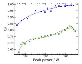
Fig. 5. Intensity correlation CS upon output peak power for LP01 (blue curve) and LP11 (green curve); dashed lines are guides for the eyes.
