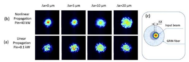
**Fig. 2.** Output beam intensity patterns versus input beam position with respect to the fiber center. (a) Linear regime, (b) nonlinear regime, (c) scheme of beam coupling (multimode GRIN fiber: 50/125, length: 3 m, input beam diameter: 36 µm - measured at 1/e2).
