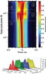
Fig. 8. Top: experimental output temporal profile upon peak power. The horizontal dashed lines represent selected peak power levels, whose corresponding waveforms are plotted in the bottom panel.
