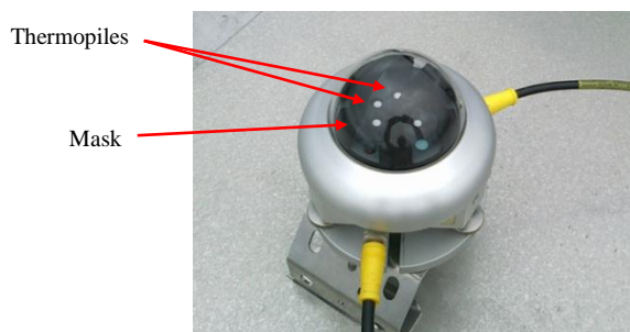
Figure 1 SPN1 sensor installed at the UKZN Howard College radiometric ground station
