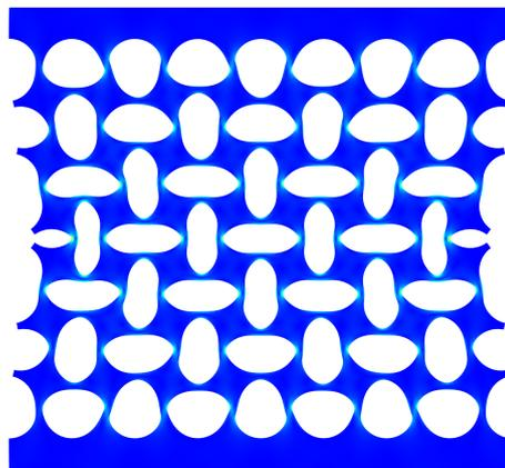
**Figure 14.** Computed deformed state of a finite  $8 \times 7$  structure. The middle cells are much more deformed than the top and bottom ones.
