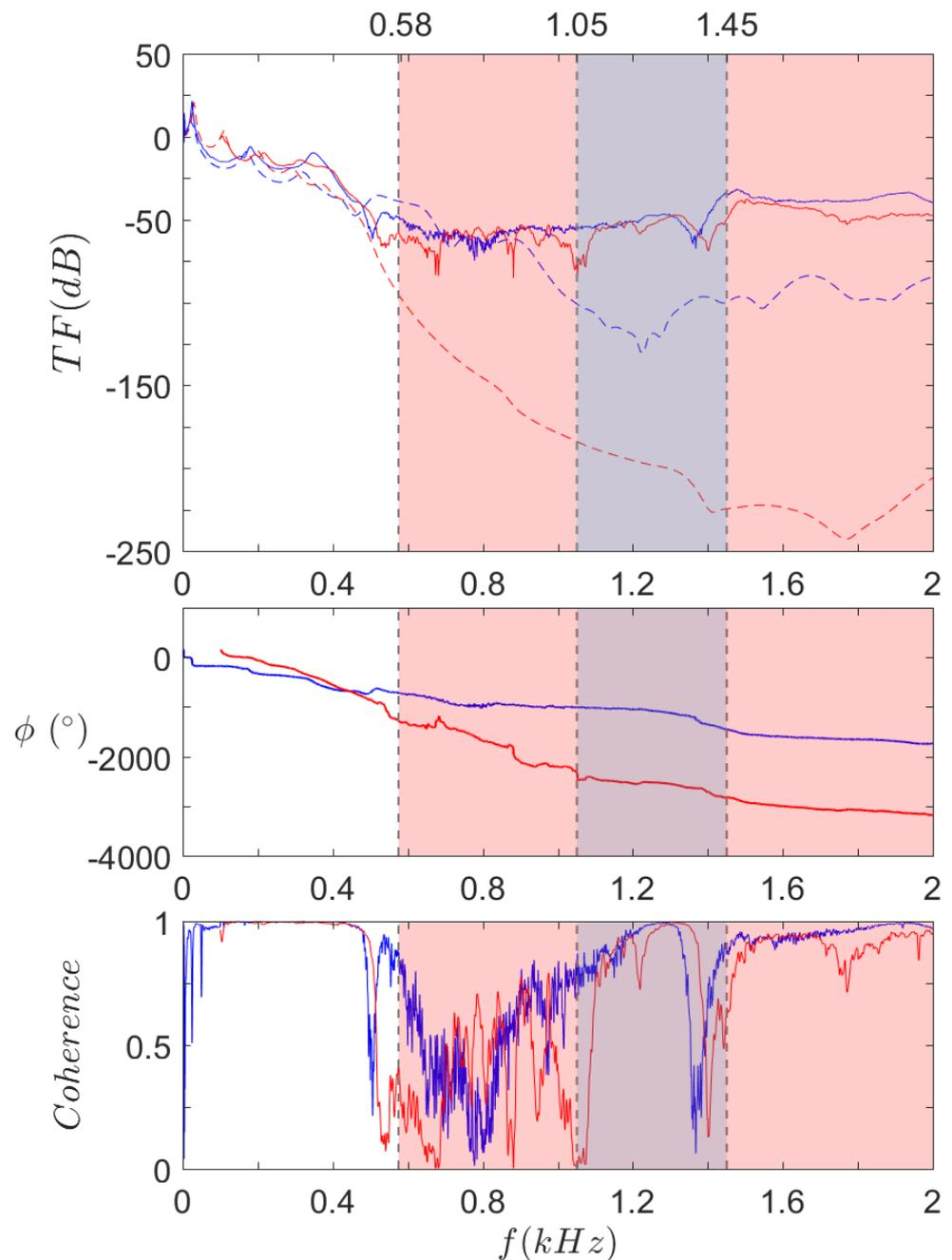
**Figure 18.** Experimental transfer functions (top), phases (middle), and coherences (bottom) of  $S_0$  and  $S_R$ , compared to their computed counterpart  $S_0$  and  $S_R$ . Omnidirectional bandgap ranges under 2 kHz for  $S_0$  and  $S_R$ , as found in the dispersion analysis.
