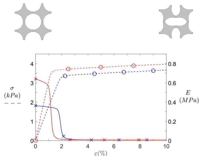
**Figure 10.** Static behaviour of  $S_0$  (blue) and  $S_R$  (red) patterns under axial compression. **-○-** Effective stress  $\sigma$  and **-×-** effective Young's modulus  $E$  against compression axis ( $Y$ ).
