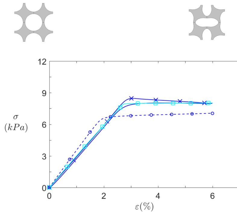
**Figure 12.** Static behaviour of  $S_0$  pattern under axial compression. Effective stresses  $\sigma$  against compression axis ( $Y$ ) for -○- infinite plates computations, -□- finite  $8 \times 7$  structures computations, and -×- experimental  $8 \times 7$  samples.
