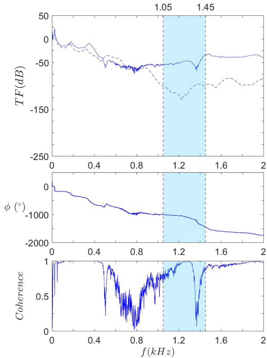
**Figure 16.** Transfer function (**top**), phase (**middle**), and coherence (**bottom**) of  $S_0$ . — Experimental and - - - computed results. ■ Omnidirectional bandgaps under 2 kHz, as found in the dispersion analysis.
