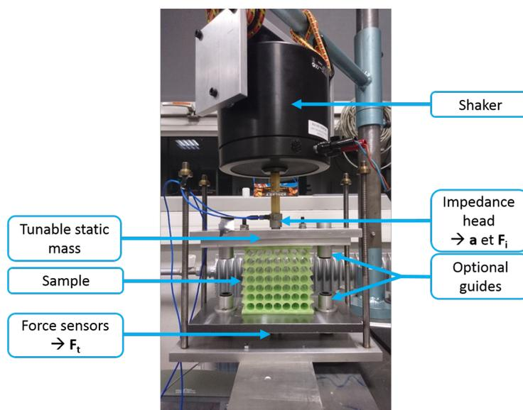
Figure 8. Test bench for vibration isolation measurements.
