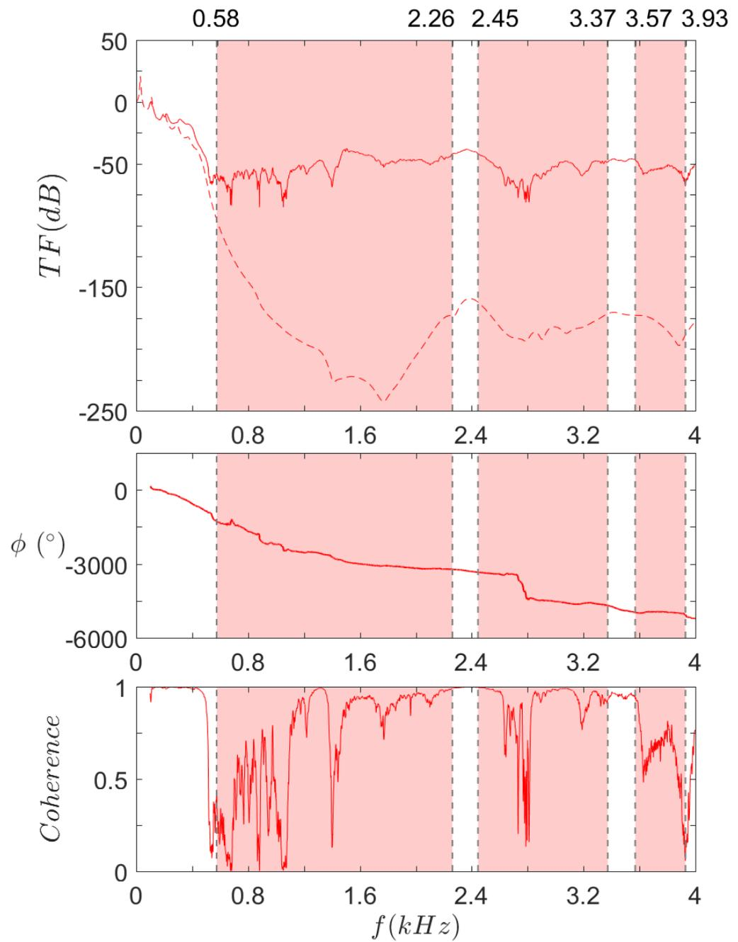
**Figure 17.** Transfer function (top), phase (middle), and coherence (bottom) of  $S_R$ . — Experimental and - - - computed results. ■ Omnidirectional bandgaps under 4 kHz, as found in the dispersion analysis.
