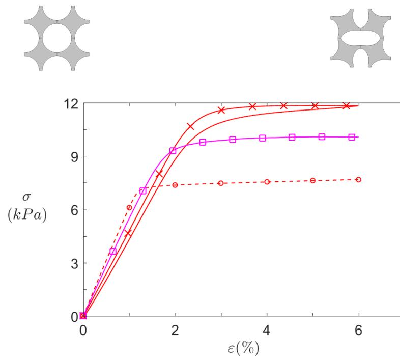
**Figure 13.** Static behaviour of  $S_R$  pattern under axial compression. Effective stresses  $\sigma$  against compression axis ( $Y$ ) for -○- 2D infinite plates computations, -□- 3D finite  $8 \times 7$  structures computations, and -×- experimental  $8 \times 7$  samples.
