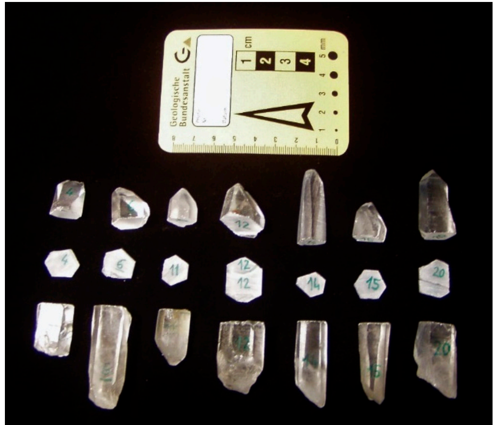
Figure 2. Some non-twinned mountain crystals with ca. 3-mm-thick sheets that were cut perpendicular to the crystallographic c-axis.
