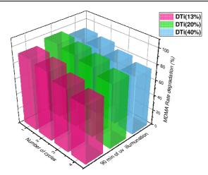
Fig.18 The reusability experiment results of MDMA degradation using DTi(13 %), DTi(20 %) and DTi(40 %)under UV-light irradiation.
