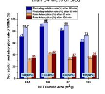
Fig. 17 Effect of the specific surface area on MDMA adsorption and photodegradation of composite contained more than 34 wt.% of SiO<sub>2</sub>.
