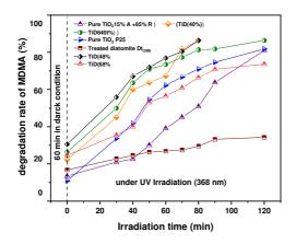
Fig. 14 Photocatalytic activity of composite containing single anatase TiO<sub>2</sub> phase (more than 34 wt.% SiO<sub>2</sub> content).
