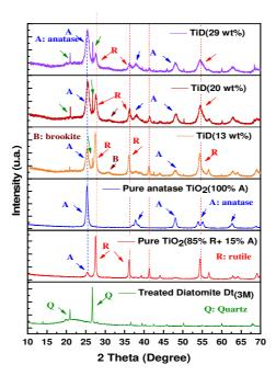
Fig. 2 XRD patterns of prepared pure anatase TiO<sub>2</sub> (100 wt. %), mixed phase TiO<sub>2</sub> (rutile:anatase is 85:15) and composite containing less than 34 wt.% of SiO<sub>2</sub>
