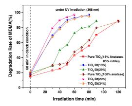
Fig. 13 Photocatalytic activity of Pure TiO<sub>2</sub> and composites prepared with small amount of diatomite (less than 34 wt.% SiO<sub>2</sub> content).
