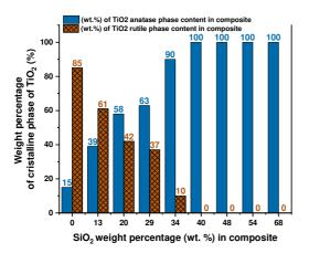
Fig. 4 Relationship between weight percentage of TiO<sub>2</sub> anatase phase and SiO<sub>2</sub> content in the composites.
