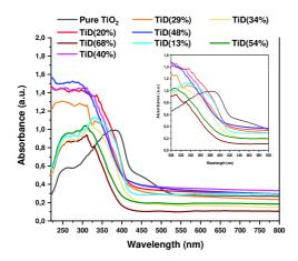
Fig. 11 The UV-Vis diffuse absorption spectra of all composite (DTi(SiO2 wt%) and pure TiO<sub>2</sub>
