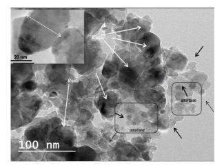
Fig. 9 TEM micrograph of pure prepared  $TiO_2$  containing 85% rutile and 15% anatase
