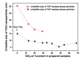
Fig. 5 Relationship between crystallite size of TiO<sub>2</sub> NPs and SiO<sub>2</sub> content in prepared composites.
