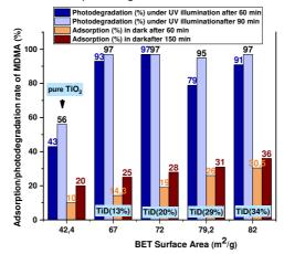
Fig. 16. Effect of the specific surface area (SAA) on MDMA adsorption and photodegradation of composite contained less than 34 wt.% of SiO<sub>2</sub>
