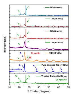
Fig. 3 XRD patterns of prepared pure anatase TiO<sub>2</sub> and composite containing more than 34 wt.% of SiO<sub>2</sub>.
