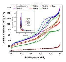
Fig. 7  $N_2$  adsorption-desorption isotherms and BJH pore size distribution plots of crude diatomite, treated diatomite  $Dt_{(3M)}$ and composite containing more than 34 wt.% of SiO<sub>2</sub>
