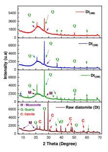
Fig. 1. XRD patterns of raw diatomite (Dt), and treated diatomites with sulfuric acid at different concentration Dt<sub>(2M)</sub>, Dt<sub>(3M)</sub> and Dt<sub>(4M)</sub>
