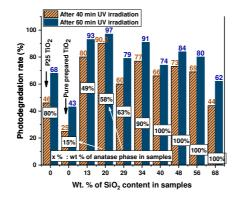
Fig 15. Effect of SiO<sub>2</sub> and anatase content on the photodegradation of MDMA after 40 and 60 min of UV irradiation (368 nm)
