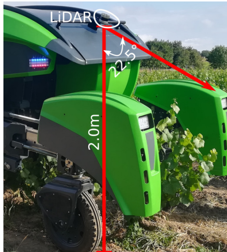
Fig. 2: LiDAR sensor's positioning.
