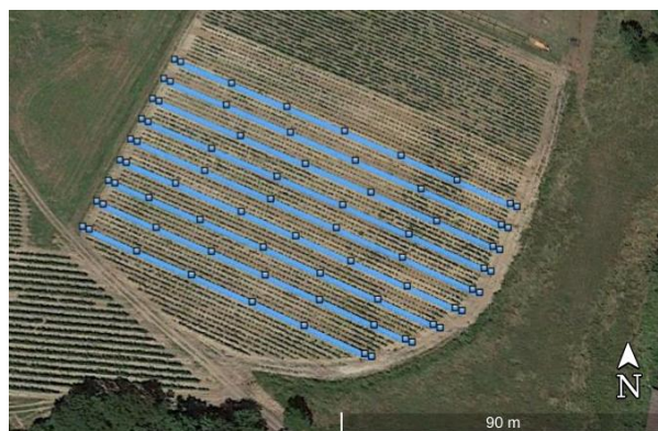
Fig. 12: Satellite image of the vineyard test field along with the geo-referenced points used to create the ground-truth path.
