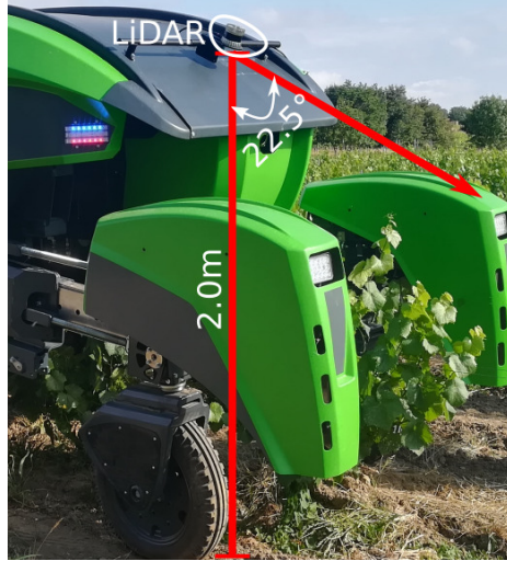
Fig. 2: LiDAR sensor's positioning.
