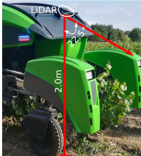
Fig. 2: LiDAR sensor's positioning.
