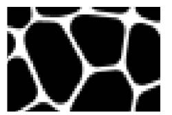
(a) Poorly resolved image of a cellular specimen (4 pixels in the micro-structure's thickness (of length equal to 0.6*mm*). The image gradient is either small (black region) or has a dominant direction (white regions).
