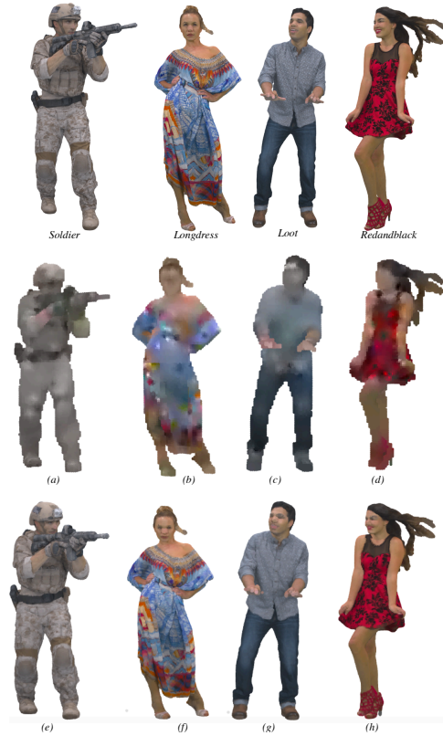
Fig. 4: Rendering results for original PCs (first row: compressed PCs using MPEG lossy PCC; second row: (a), (b), (c), (d) and using our optimized TSPLVQ; third row: (e), (f) (g), (h)).
