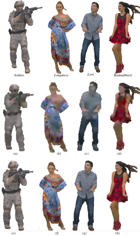
Fig. 2. Rendering results for original point clouds (first row), compressed point clouds using MPEG lossy PCC (second row): (a), (b), (c), (d) and using our optimized TSPLVQ (third row): (e), (f) (g), (h).
