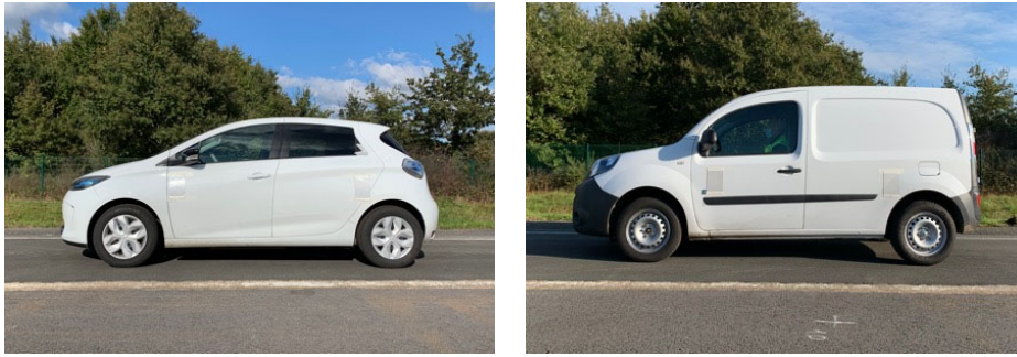
Figure 9 – Two tested EV models: Renault ZOE fitted with Michelin Energy EV 185/65 R15 tyres (left) and Renault KANGOO Z.E. fitted with Michelin Energy Saver 195/65 R15 tyres (right).
