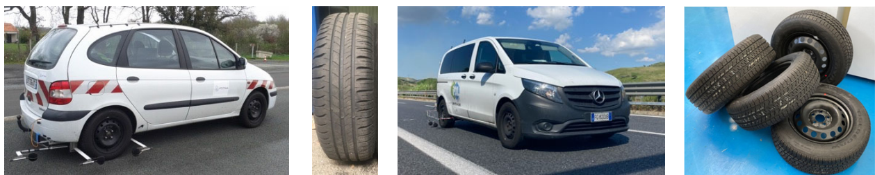
Figure 7 – CPX test vehicles: Renault Scénic fitted with Michelin Energy Saver tyres (left) and Mercedes Vito fitted with SRTT tyres (right).
