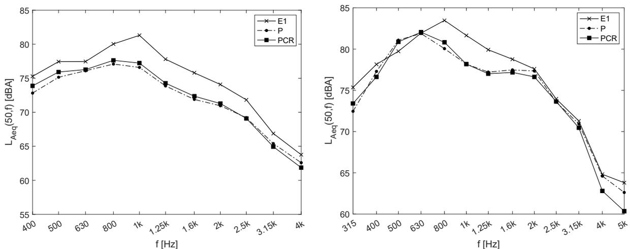
Figure 8 – CPX noise spectra for the Michelin Energy Saver 195/60 R15 tyre (left) and for the SRTT P225/60 R16 tyre (right) at the reference speed of 50 km/h.
