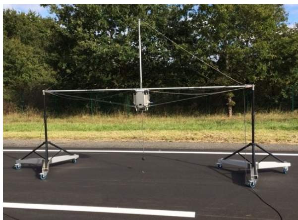
Figure 5 – Sound absorption measurement system (left) and sound absorption coefficient in one-third octave bands (right) measured on prototype road surfaces P and PCR.
