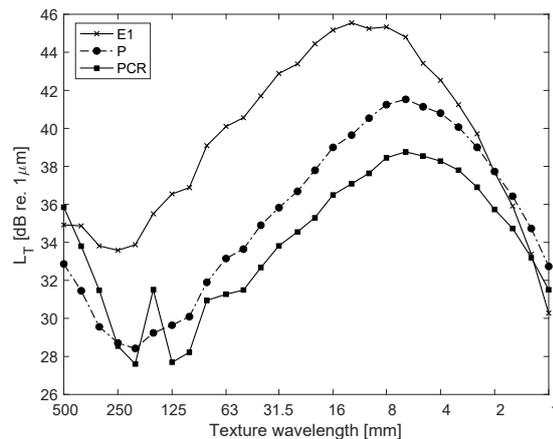
Figure 4 – 3D profilometer (left) and surface texture spectra measured on the 3 test sections (right).
