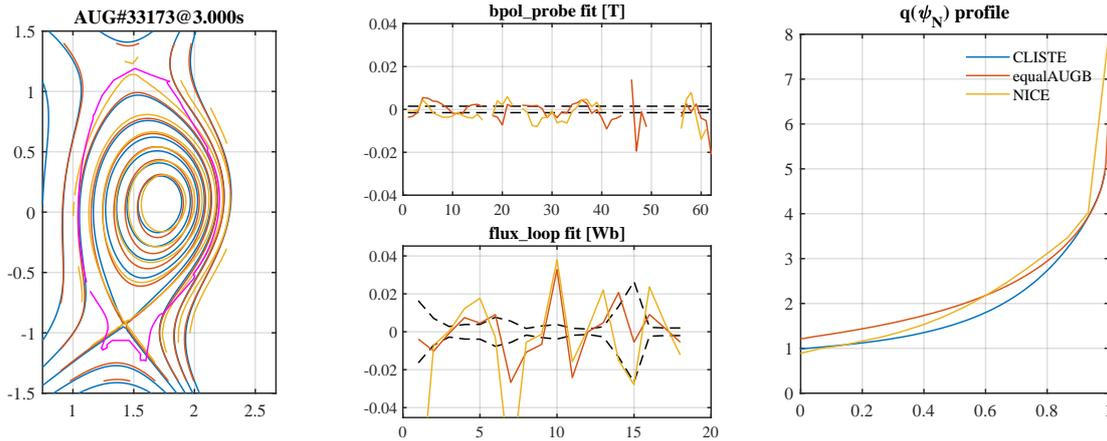
Figure 3: Comparison of flux contours, magnetic probe and flux loop reconstruction errors and obtained  $|q|$  profiles for the codes CLISTE, EQUAL and NICE using data from AUG discharge 33173 at  $t = 3.0$ s. Note that the reconstruction errors for CLISTE are missing since this data hasn't been mapped to IDS format.
