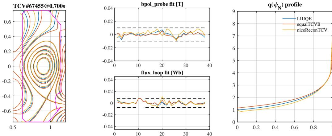
Figure 1: Comparison of flux contours, magnetic probe and flux loop reconstruction errors and obtained  $|q|$  profiles for the codes LIUQE, EQUAL and NICE using data from TCV discharge 67455 at  $t = 0.7$  s. Black dashed lines indicate the absolute error for the different signals.
