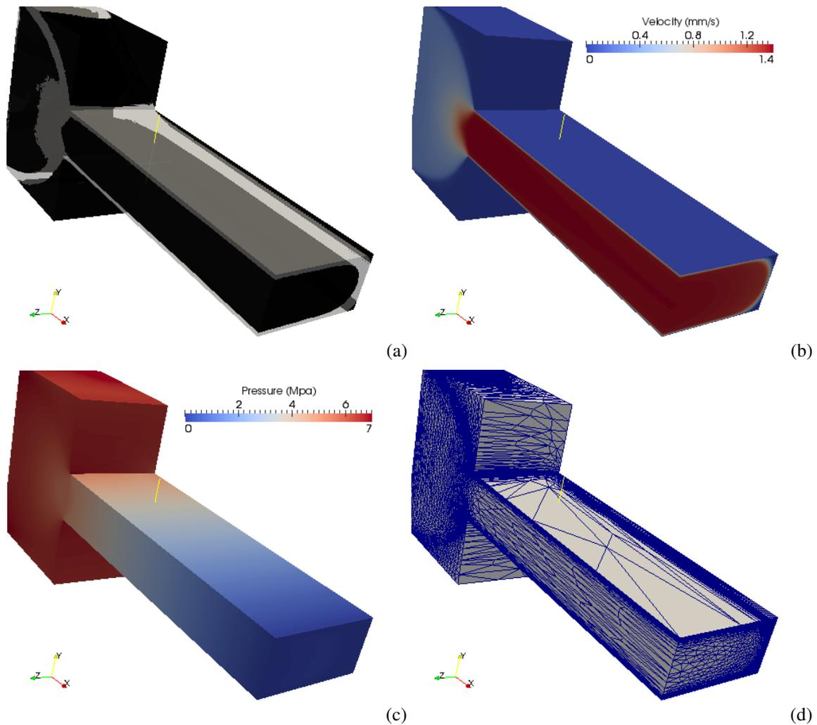
FIG. 1 – 3-D simulation results (symmetry plane is on the left face). (a) Unyielded zones (in black) produced by a Bingham fluid inside a rectangular die. (b) Norm of the velocity field. (c) Pressure field. (d) Adapted mesh. It can be noticed that the undeformed zones in the die occupy most of the region and the flow is mostly a plug.
