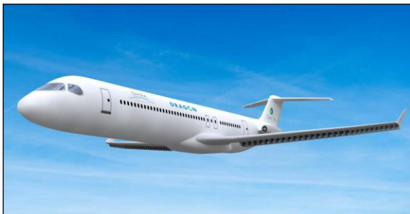
Fig. 1: Illustration of the DRAGON concept (configuration including 40 electric motors).
