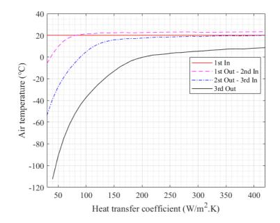
Figure 20: Air temperature going through the three air stage expanders as a function of heat transfer coefficient
