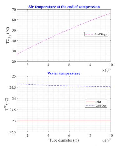
Figure 28: Air/water temperature at the end of compression function of 2<sup>nd</sup> stage compressor tube diameter
