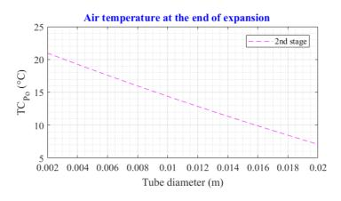
Figure 31: Air temperature at the end of expansion function of 2<sup>nd</sup> stage expander tube diameter
