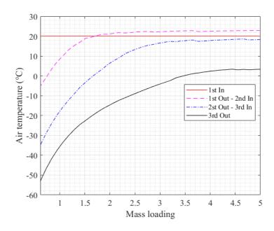
Figure 24: Air temperature as a function of mass loading
