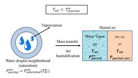
Figure 34: Mass transfer between water droplets injected inside the cylinder during expansion
