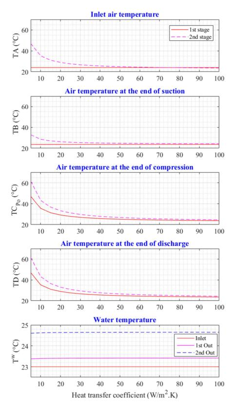
Figure 26: Air/Water temperature at different air compression states function of the heat transfer coefficient. The legend of the first figure at the top has to be considered for the other figures below.
