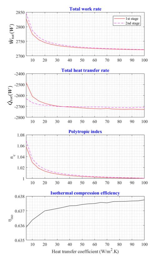
Figure 27: Several liquid piston compressor model outputs function of the heat transfer coefficient
