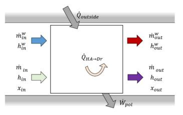
Figure 9: Conservation of energy for a steady-flow, open system
