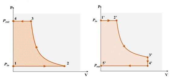
Figure 10: PV diagram of the air compression (left) and expansion (right) cycles
