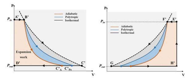
Figure 12: PV diagram of the air (left) and water (right) expansion cycle
