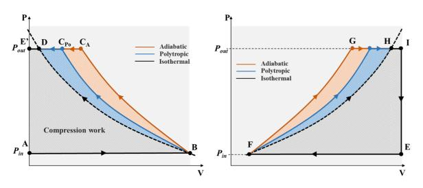
Figure 11: PV diagram of the air (left) and water (right) compression cycle
