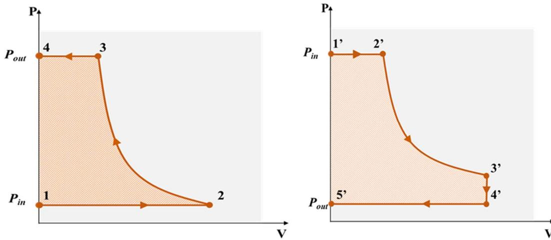
Figure 10: PV diagram of the air compression (left) and expansion (right) cycles
