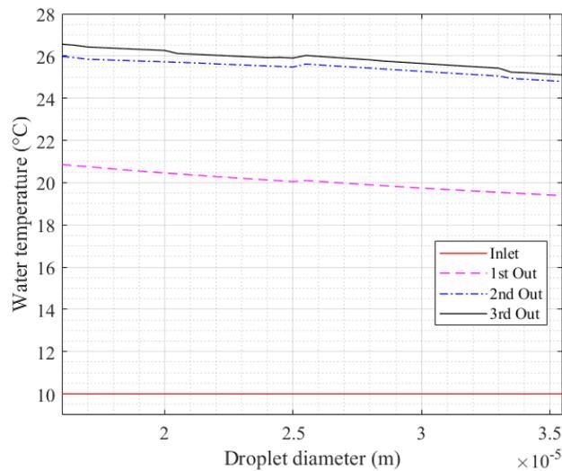
Figure 17: Water temperature as a function of water droplet diameter
