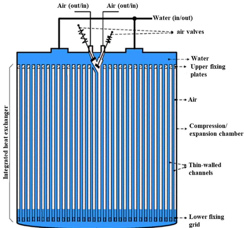
Figure 4: Energy conversion chamber developed by Enairys Powertech [21]
