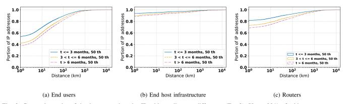
Fig. 3: Comparing pairs of database snapshots by IP address distance difference (Eq. 3). Up to 22% of addresses move more than 40km among snapshots in a three month window.
