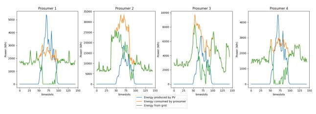
FIGURE 3. CONSUMPTION, PRODUCTION AND IMPORT FOR THE PV ONLY SCENARIO
