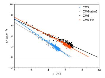
**Figure 1.** Scatterplot of the global-mean surface-air temperature response  $(\Delta T_s, \text{unit: K})$  and net TOA radiative imbalance  $(\Delta R, \text{unit: W.m}^{-2})$  in the CNRM-CM abrupt-4×CO<sub>2</sub> experiments: CNRM-CM5 (blue), CNRM-CM6-atm5 (gray), CNRM-CM6-1 (black), and CNRM-CM6-1-HR (red).
