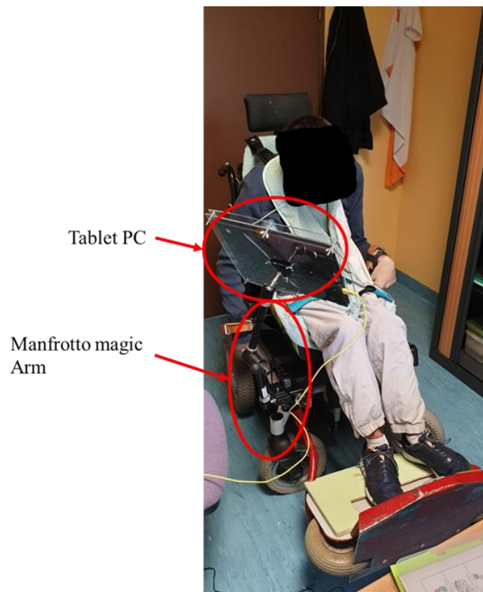
Fig. 13. Integration of the interface in the wheelchair environment.
