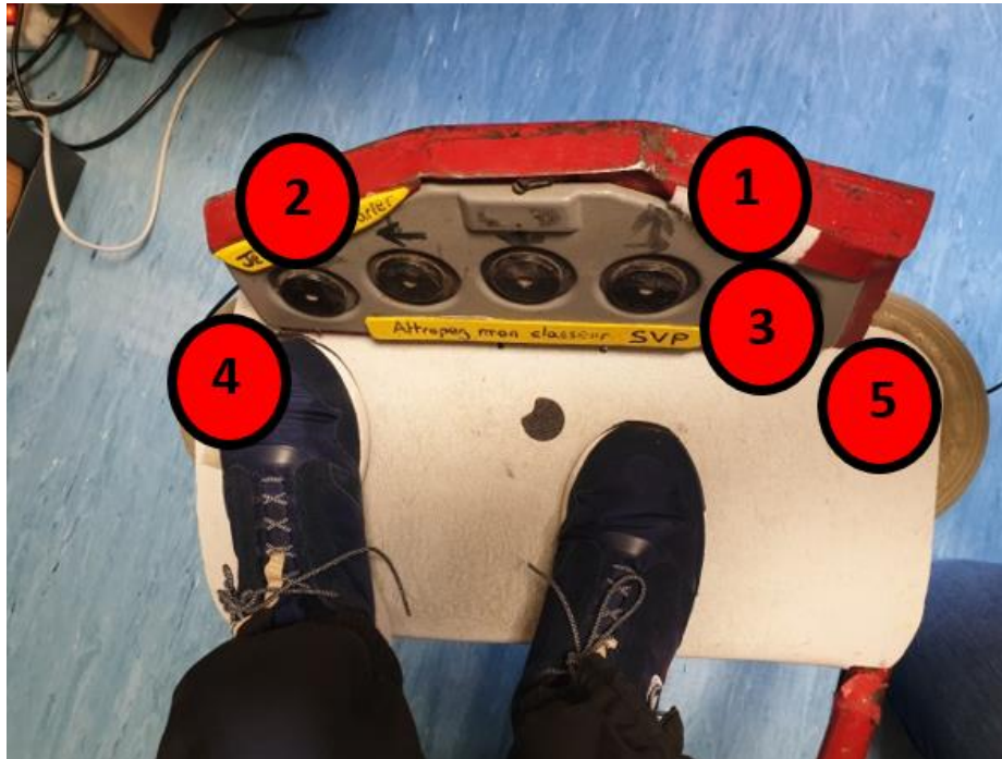
Fig. 6. Various switch positions to control the AAC interface.
