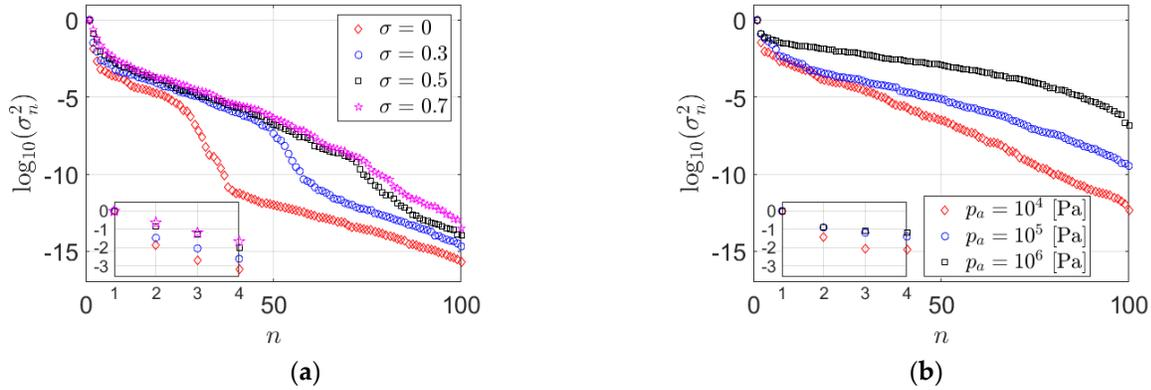
**Figure 2.** (a) PCA variance obtained with  $L_2$ , for various values of polydispersity of bubble clouds with  $B = 5$ . (b) PCA variance obtained with  $L_2$ , for polydisperse bubble clouds with  $B = 5$  excited by various amplitudes of the external pressure.
