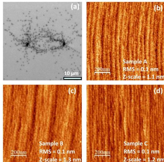
**Figure 1:** (a) A cathodoluminescence image of two clusters on a GaN substrate. (b), (c), (d) Surface morphology analysed by atomic force microscopy in a scan range of  $2 \times 2 \mu\text{m}^2$  for the A, B and C samples, respectively. The root mean square roughness was estimated to about 0.1 nm for all the samples.
