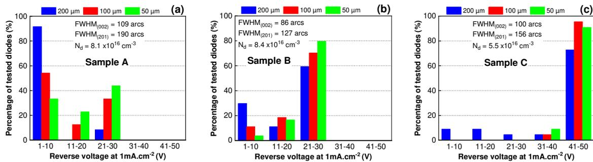
**Figure 6:** (a), (b), (c) Histogram of percentage of tested diodes against the reverse breakdown voltage at the current density of  $1 \text{ mA.cm}^{-2}$  for diodes fabricated on the samples A, B and C, respectively. XRD data and donor concentrations are also recalled.
