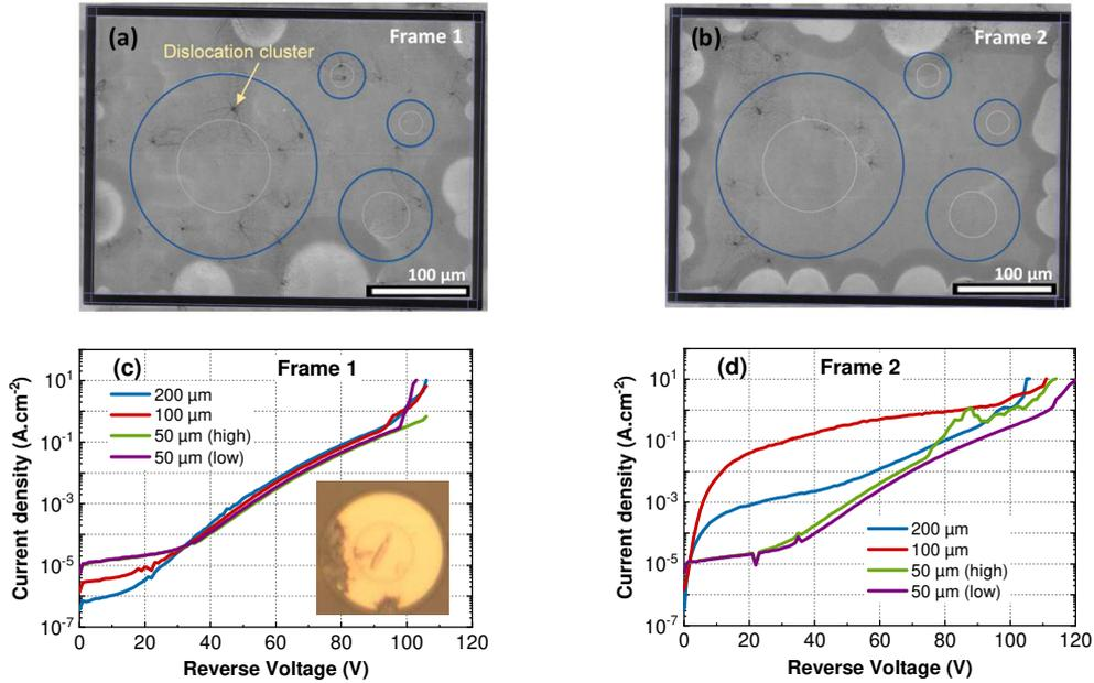
**Figure 5:** (a), (b) Cathodoluminescence images of GaN layer within Ni frames of sample C: blue circles represent locations of the diodes. (c), (d) Plots of reverse current-voltage characteristics of diodes fabricated within the frame 1 and frame 2, respectively. The inset of figure (c) shows an optical microscope image of the 100  $\mu\text{m}$  diode damaged by the hard breakdown.
