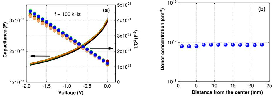
**Figure 3:** (a) Solid lines represent capacitance-voltage curves and dotted lines show the  $1/C^2$  – voltage profiles. The measurement is recorded at the frequency  $f = 100 \text{ kHz}$ . (b) Donor concentration profile of  $200 \mu\text{m}$  diodes along the radius of sample A.
