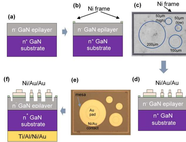
**Figure 2:** Schematic diagram of the device processing.
