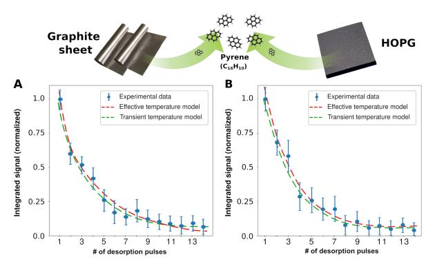
Figure 5: Experimental datapoints (four-zone average) recorded with the "signal decay" approach for pyrene desorbing from (a) graphite sheet ( $F_{des} = 50 \text{ mJ cm}^{-2}$ ) and (b) HOPG ( $F_{des} = 61 \text{ mJ cm}^{-2}$ ). Steady-state (red dashed line) and transient (green dashed line) decay curves calculated with parameters from Table 3.
