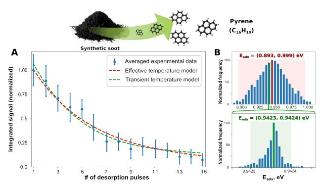
Figure 4: (a) Steady-state (red dashed line) and transient (green dashed line) models fitted to the signal decay curve (four-zone average experimental datapoints) of pyrene desorbing from activated carbon ( $F_{des} = 32 \text{ mJ cm}^{-2}$ ). The plotted fits correspond to the maximum (mode) of the Bayesian posterior distributions shown in (b) – top: steady state, bottom: transient. Shaded areas represent the 95% credibility intervals of  $E_{ads}$ .
