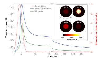
Figure 3: Temporal evolution of the temperature in the center of the irradiated spot T(x = 0, y = 0, z = 0, t) calculated for nano-porous soot (blue lines) and graphite (green lines) obtained for  $F_{des} = 32 \text{ mJ} \text{ cm}^{-2}$ . The temporal profile of the desorption laser is plotted for comparison (red dashed line). Snapshots of the radial distribution of the temperature at various delays after the laser pulse are presented in the inset.
