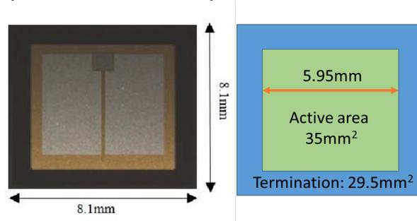
**Fig. 1:** 6.5kV commercial device picture and evaluation of its respective active and termination area
