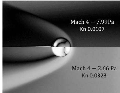
Figure 6: Shock wave positions: comparison of the experimental shock wave position obtained at Mach 4 – 2.66 Pa with the position given by the empirical relation of Billig (Eq. 1) around a 40 mm-diameter sphere (left panel), and comparison of the standoff distance obtained with a 5 mm-diameter sphere in a Mach 4 – 7.99 Pa flow (top) and in a Mach 4 – 2.66 Pa flow (bottom).
