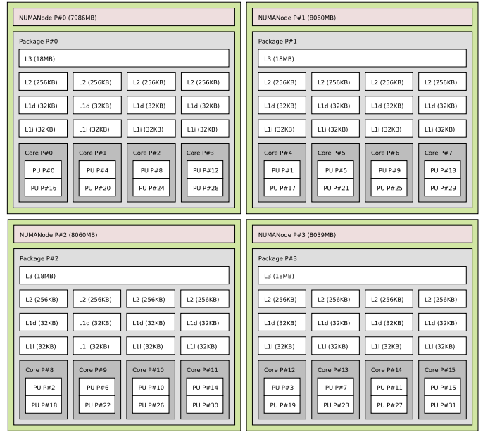
Fig. 1. Mid-end host server: Dell PowerEdge R910 (1stopo picture).
