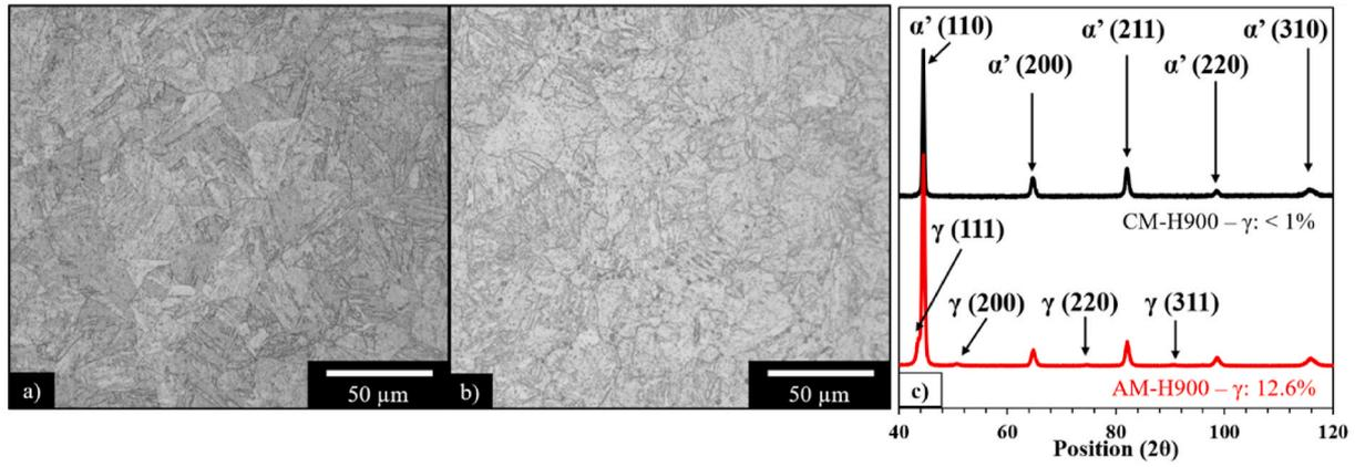
**Fig. 1.** Observations using an Axiovert A1m Zeiss optical microscope, after chemical etching of the a) CM-H900 and b) AM-H900 samples. c) Experimental X-ray diffractograms obtained using a Bruker D8 GIXRD machine with a Cu anticathode for the AM-H900 and CM-H900 samples. (Color online only; two columns). (For interpretation of the references to colour in this figure legend, the reader is referred to the Web version of this article.)
