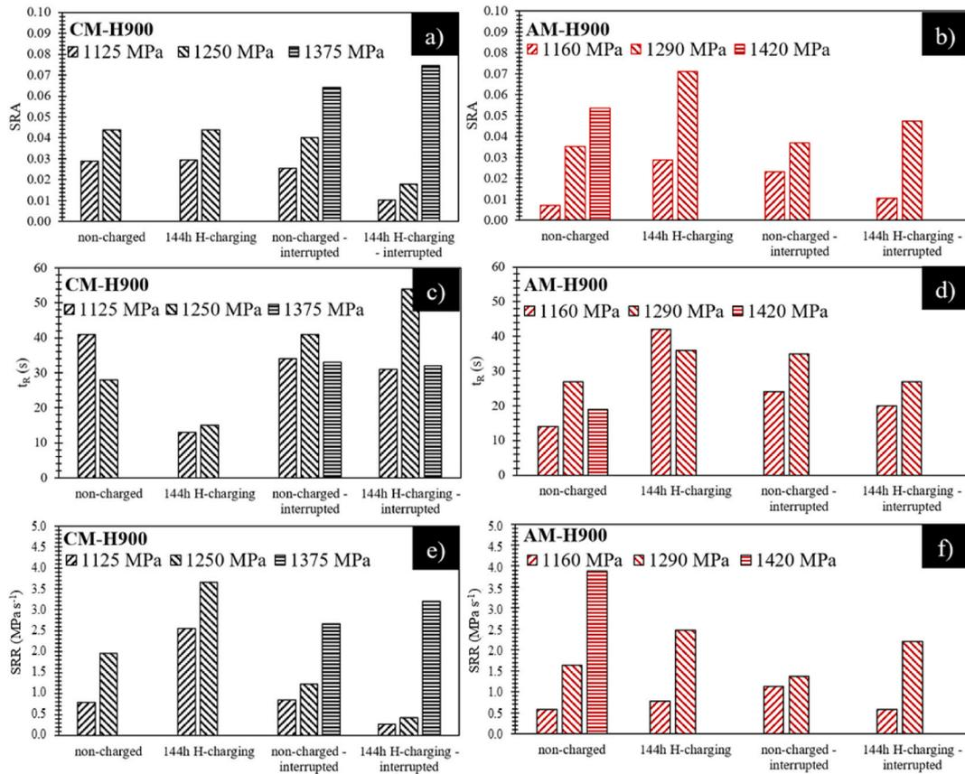
**Fig. 13.** SRA as calculated by Equation (2), critical time  $t_R$  as defined in Fig. 3 [21], and SRR as given by Equation (3), for the (a, c, and e) CM and (b, d, and f) AM samples. Results are for the non-charged and 144 h hydrogen-charged samples, for both the non-interrupted and interrupted tests (stress-holding step at 300 MPa for 168 h). (Color online only). (For interpretation of the references to colour in this figure legend, the reader is referred to the Web version of this article.)
