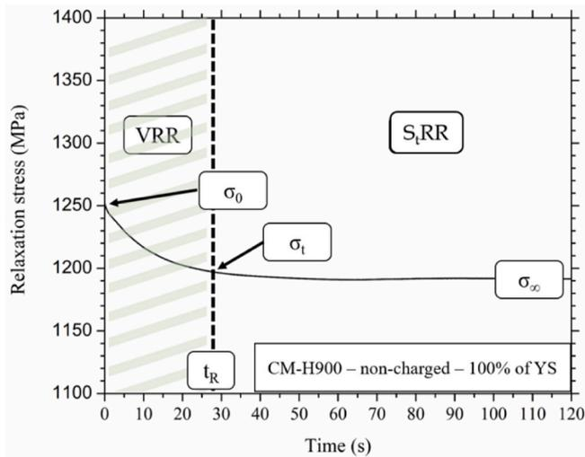
**Fig. 3.** Schematic of a relaxation curve. VRR and  $S_tRR$  regimes are identified using the threshold stress  $\sigma_t$  given by Equation (1) and the critical time  $t_R$  [21].  $\sigma_0$  is the initial relaxation stress, and  $\sigma_\infty$  is the stress at the end of the relaxation period. (Color online only).
