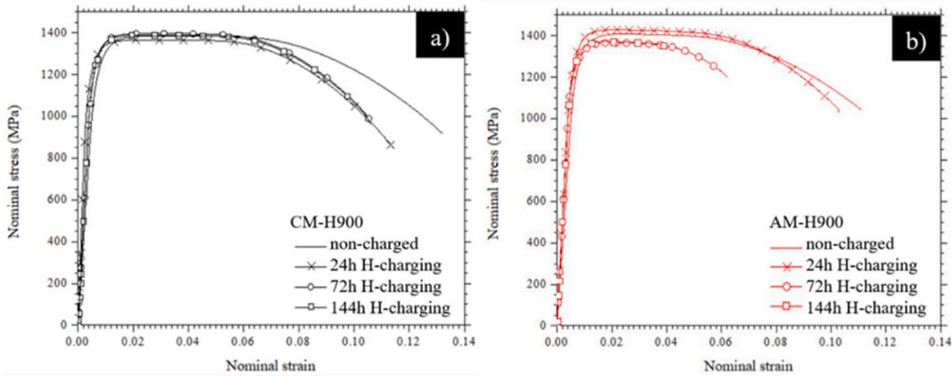
**Fig. 6.** Tensile curves for the a) CM and b) AM samples at different hydrogen-charging durations. The tensile curves plotted for the non-charged samples are also indicated for comparison. (Color online only). (For interpretation of the references to colour in this figure legend, the reader is referred to the Web version of this article.)
