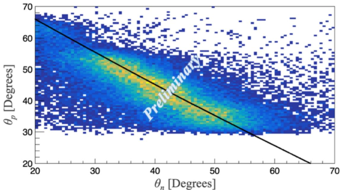
**Figure 2.** Correlations between the polar angles of the recoil proton and recoil neutron ( $\theta_p$ ,  $\theta_n$ ) in the present measurement. The black solid line indicates the correlation pattern from the kinematical calculation.
