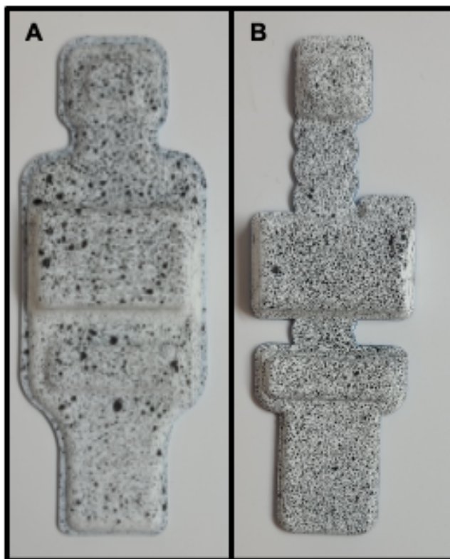
1 2 3 4 5 6 7 8 9 10 11 12 13 14 15 16 17 18 19 20 21 22 23 24 25 26 27 1 28 2 29 3 Figure S3. Speckle patterns on unoptimized and optimized designs for DIC experiments. The 4 30 black speckles, size of \sim 200\text{-}500\ \mu\text{m} , were coated on the devices by the spray-painting 31 method. 32 5 33 6 34 7 35 8 36 9 37 10 38 11 39 12 40 13 41 14 42 15 43 16 44 17 45 18 46 19 47 20 48 21 49 22 50 23 51 24 52 25 53 26 54 55 56 57 58 59 60 61 62 63 64 65
